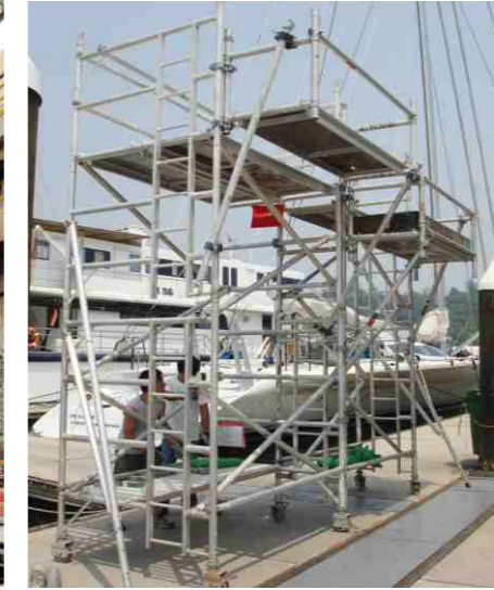
Special tower for yacht maintenance
